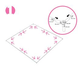
First connect the top straight horizontal tubes (Blue Colored Label: T) and corner connectors. Snap them together.
