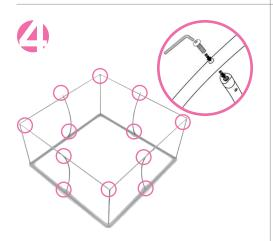
Locate each screw holes on the sides of the top and bottom tubes. Align the vertical curve tubes within the screw holes at each end. Make sure the middle tubes are bowing inward. Insert large screws into the top and bottom screw holes. Also insert eyehook screws into the top corner connectors. Tighten to secure.
