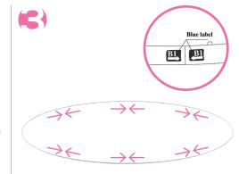
Then connect the bottom curve horizontal tubes (Blue Colored Label: B) and snap them together.
