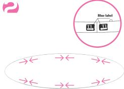
• First connect the top curve horizontal tubes (Blue Colored Label: T) and snap them together.
