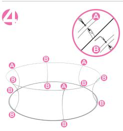
Locate each screw holes on the sides of the top and bottom tubes. Align the vertical curve tubes within the screw holes at each end. Make sure the middle tubes are bowing inward. Insert eyehook (A) and large screws (B) into the top and bottom screw holes. Tighten to secure.
